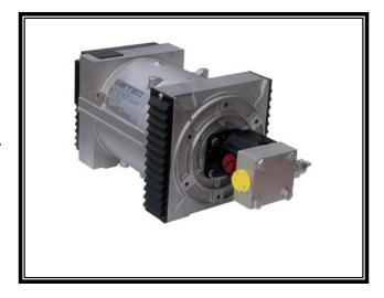
**Overall Efficiency** 81 % **Operating Speed 3600 RPM Minimum Flow 7.5 GPM Ideal Flow** 9 GPM **Maximum Flow 15 GPM** Free Air Flow 7 cfm **Recommended Filtration** 10 m **Max.Oil Temperature** 180 F **Recommended Tank Size** 20 Gal.
