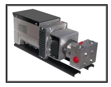
**Overall Efficiency** 86 % **Operating Speed 3600 RPM Minimum Flow 12 GPM Ideal Flow 15 GPM Maximum Flow 40 GPM** Free Air Flow 11 cfm **Recommended Filteration** 10 m Max.Oil Temperature 180 F Min.Tank Size 30 Gal.
